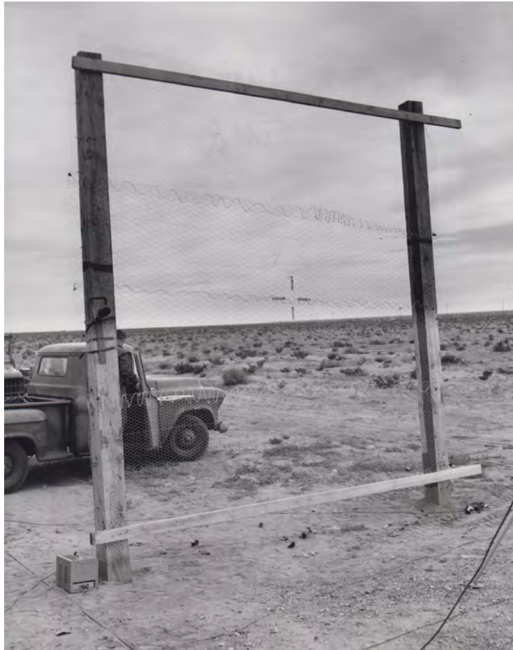
Figure 35. Some targets used for the Shillelagh testing were simple wood frames filled with wire mesh (US Army photo, courtesy Jack Dage).
