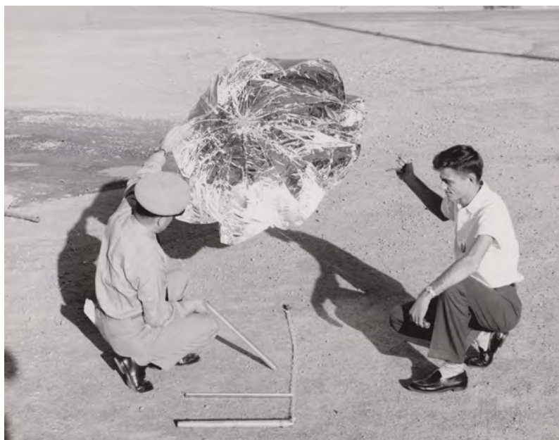
Figure 54. The reflective metallic parachute that was deployed as a radar target by the Loki-Dart sounding rocket ( US Army photo ).
