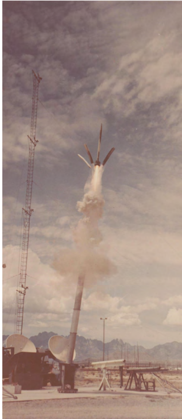
Figure 55. An ARCAS launch from the ASL launch area circa late 1960s or early 1970s. The three panels detaching from the rocket are plastic sleeves that sealed the rocket within the launcher tube (US Army photo).
