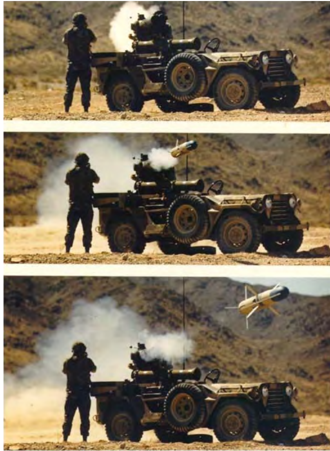
Figure 38. Photo sequence of a jeep mounted TOW launch (US Army photo).
