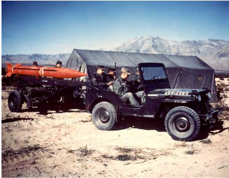
Figure 20. The Little John was a portable system that was easily towed by a Jeep (US Army photo).
