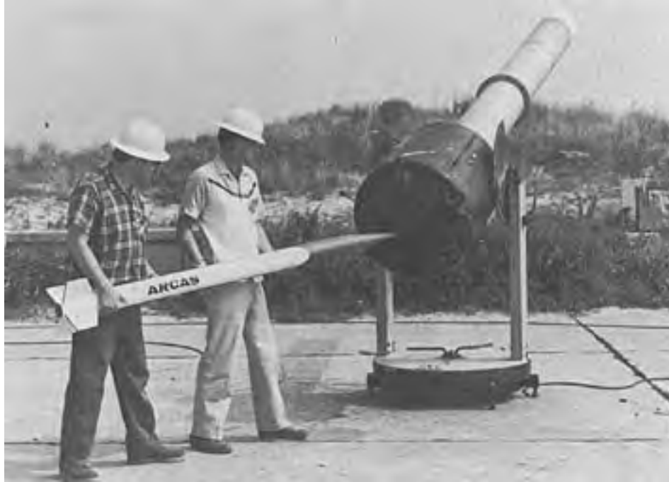
Figure 56. Technicians load the ARCAS rocket into its launcher, showing the breech loading operation of the system ( photo courtesy NASA ).
